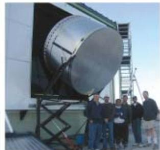
Drum for uniform illumination of each fluorescence camera – part of end to end calibration .
